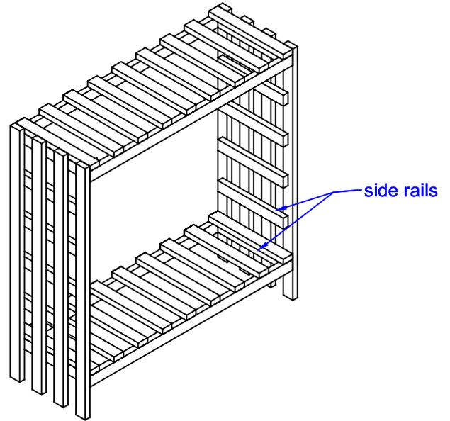
3. Keep adding shelves from the bottom up and nailing them on. Securing the top last.
