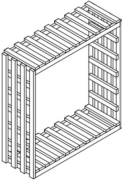
2. Nail only the bottom shelf to the side rail. Leave the top shelf to keep the spacing.
