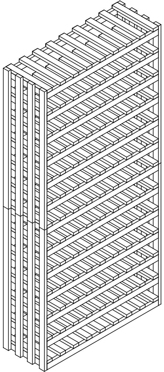
6. Anchor the racks to the wall using the recommended hardwares (not provided)
