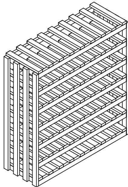
5. Middle Stack and Top Stack rack can be place directly on top.
